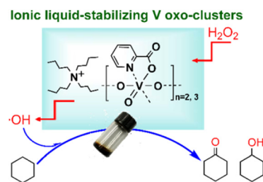
Fig. 4 IL-stabilized vanadium oxo-clusters catalyzing alkane oxidation. Adapted from ref. 63 with permission from Royal Society of Chemistry, copyright 2020.
