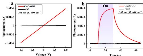
Fig. 4 (a)  $I$ - $V$  characteristics and (b)  $I$ - $t$  measurements of rGO and 2D CuO/rGO photodetectors under exposure to 395 nm light.
