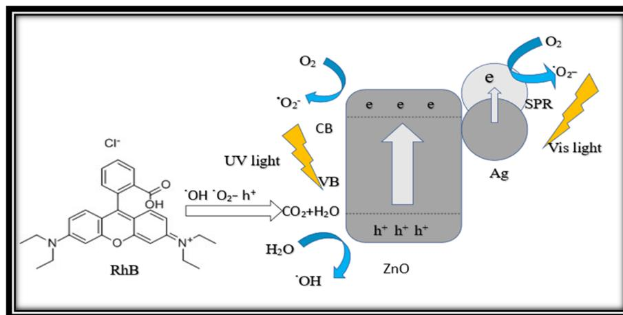
Fig. 17 Illustration of photocatalytic process of Ag@ZnO@C.
