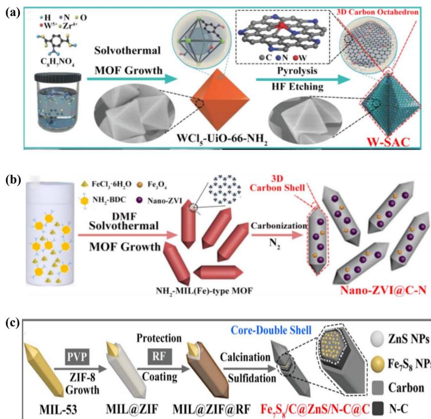
Fig. 12 (a) Synthesis of MOF-derived 3D polyhedral W-SAC.<sup>134</sup> (b) Synthesis of MOF-derived 3D polyhedral nano-ZVI@C-N.<sup>135</sup> (c) Preparation of 3D core-shell  $\text{Fe}_7\text{S}_8/\text{C}@Zn\text{S}/\text{N-C}@C$ .<sup>136</sup>
