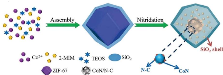
Fig. 18 Synthetic procedure of yolk-shell CoN/N-C@SiO<sub>2</sub> nanomaterials with dual active sites.<sup>79</sup>
