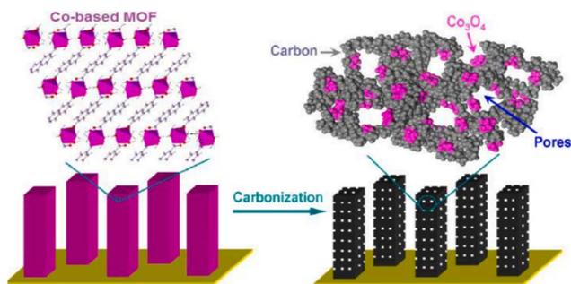
Fig. 8 Carbonization process of Co-based MOF into  $\text{Co}_3\text{O}_4$ -carbon nanowire arrays.<sup>72</sup>
