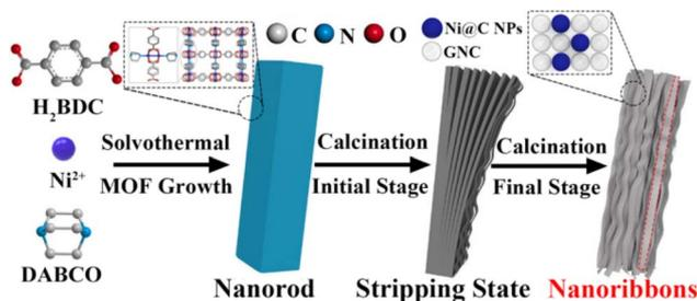
Fig. 10 Stepwise synthesis of MOF-derived 2D carbon nanoribbons.<sup>124</sup>
