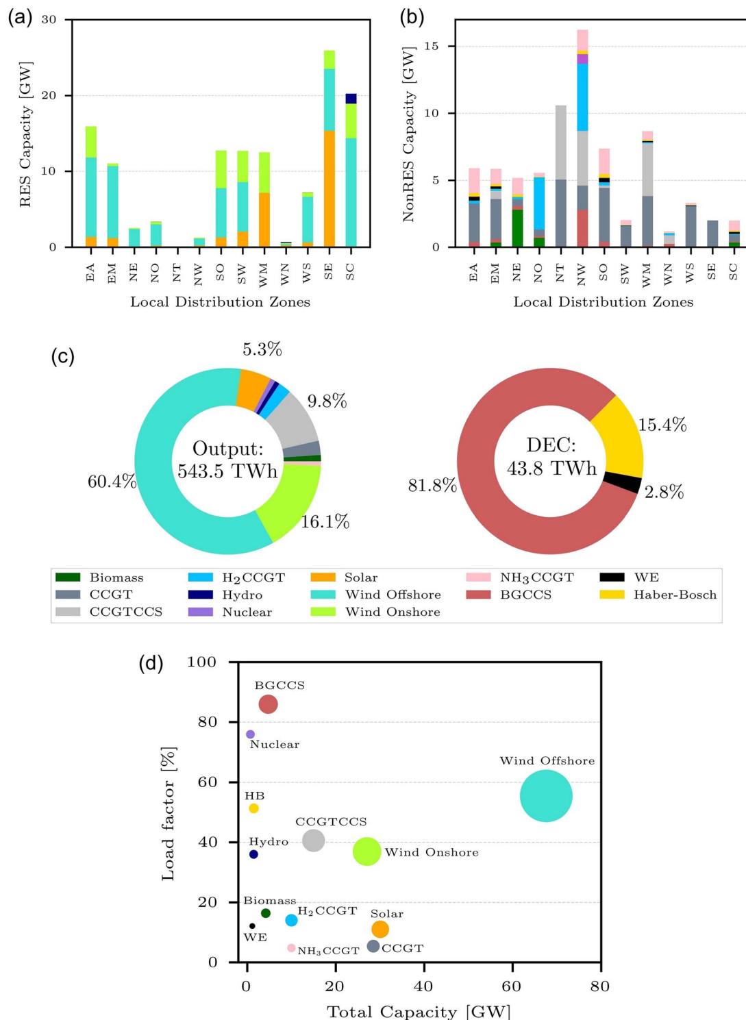
Fig. 9 Planning decisions and operation indicators for GB's power system in 2040: (a) capacity allocation of renewable technologies, (b) capacity allocation of non-renewable technologies (c) electricity generation & DEC production mix, (d) load factors in 2040 (sizes are representative of the relative total generation).
