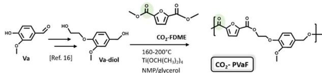
Fig. 7 Synthesis of Va-diol: (2-(4-(hydroxymethyl)-2-methoxyphenoxy) ethanol) from vanillin and polycondensation with CO<sub>2</sub>-FDME to obtain the CO<sub>2</sub>-based biopolyester (CO<sub>2</sub>-PVaF).
