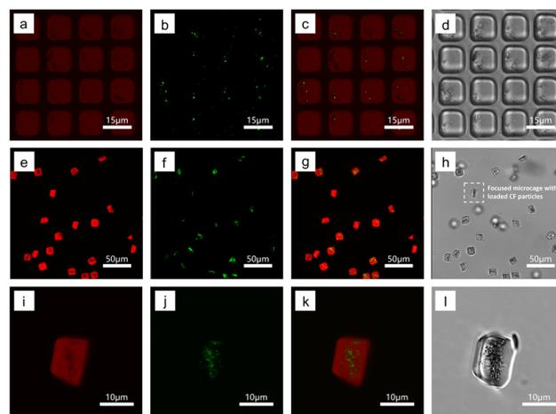
**Fig. 3** CLSM images of PLA microcages confirm the encapsulation of CF model drug. (a–d) CF loaded PLA microcages printed and embedded inside the microwell array of patterned PDMS stamp. (e–h) CF loaded printed PLA microcages dispersed in DI water. (i–l) Higher magnification of (e–h) focused on a single PLA microcage. PLA is labelled with red fluorescent dye Nile Red and the green color represents the encapsulated CF.
