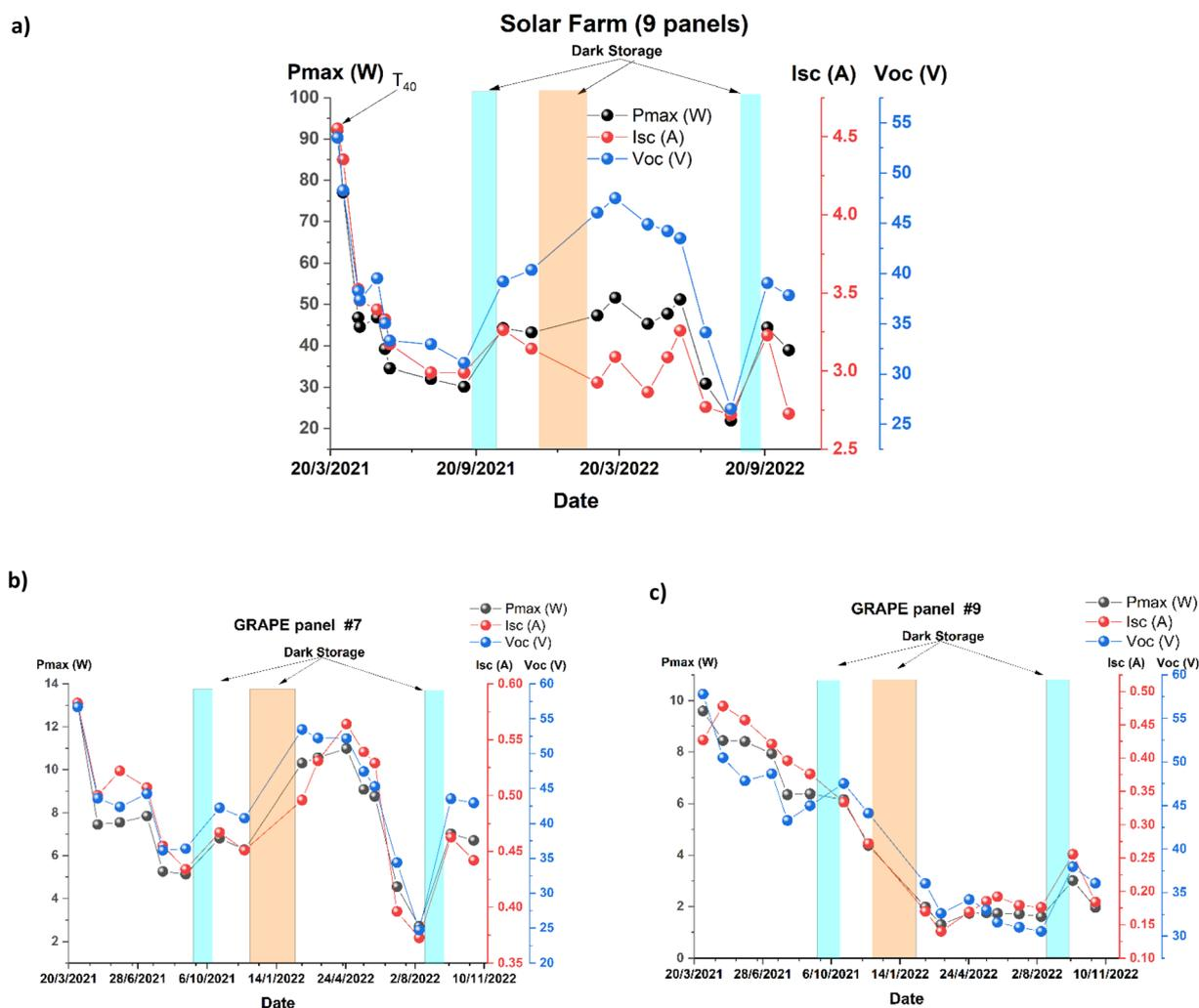
Fig. 4 Electrical parameters ( $P_{max}$ ,  $I_{sc}$ , and  $V_{oc}$ ) extracted from the  $I$ - $V$  characteristics of (a) solar farm, (b) GRAPE panel #7, and (c) GRAPE panel #9 for the period 2021–2022. In graphs a, b and c, dark storage periods are highlighted with (a) cyan (1 month DS period applied twice), (b) orange (3 month DS period applied once).
