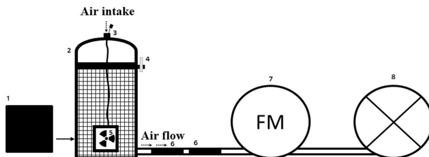
Fig. 1 Scheme of apparatus used for measurement of  $K_{TA}$  of AAs; 1- textile pieces before wrapping to the chamber mesh (Fig S1<sup>†</sup>), 2- glass chamber with a ground joint lid, mesh and airtight seal, 3- steel capillary pierced through a septum for air intake, 4- metal clamp, 5- small fan, 6- two glass tubes filled with Tenax adsorbent, in series, 7- air mass flow meter, 8- low volume air pump.
