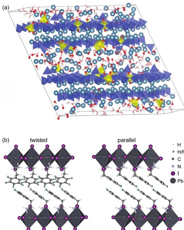
**Fig. 7** (a) Representative atomic-level structure of zinc-modified C-S-H as determined with a Zn:Si ratio of 0.15. Silicate tetrahedra are depicted in blue; zincate tetrahedra are depicted in yellow; and calcium ions are depicted in light blue.<sup>159</sup> and (b) the structure of S<sub>2</sub>PbI<sub>4</sub> layered perovskites with twisted (left) and parallel (right) relative orientations of the aromatic rings in adjacent layers.<sup>160</sup> Adapted from ref. 159 and 160.
