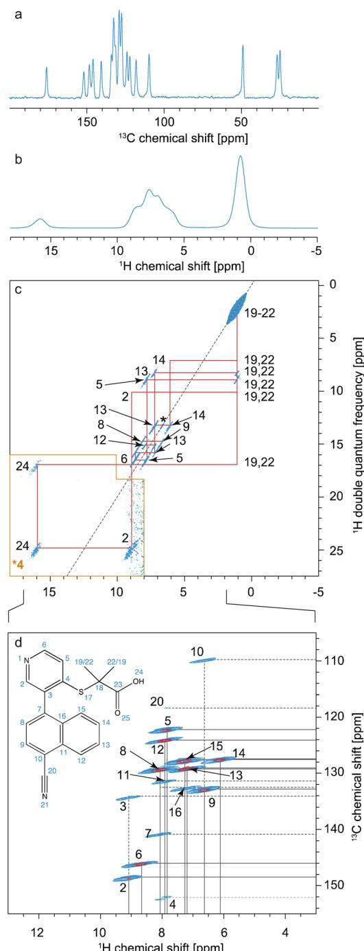
**Fig. 13** Spectra used for the <sup>1</sup>H detection based assignment of Verinurad (chemical structure shown inset).<sup>128</sup> (a) 1D <sup>1</sup>H spectrum at 160 kHz MAS. (b) <sup>13</sup>C CP spectrum at 100 kHz MAS. (c) 2D <sup>1</sup>H-<sup>1</sup>H BABA spectrum obtained at 160 kHz MAS. Red lines indicate the connectivities between cross peaks. (d) The aromatic region of the 2D hCH long-range spectrum in blue (4 ms direct CP contact time) overlaid with a 2D hCH short-range
