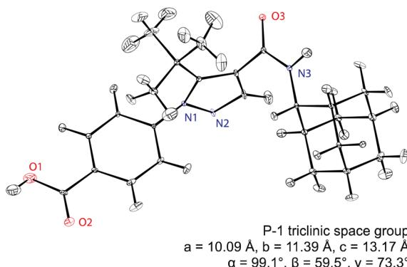
Fig. 5 The *de novo* structure of AZD8329 determined by  $^1\text{H}$  chemical shift driven NMR powder crystallography.<sup>55,57,217</sup> Adapted from ref. 57.
