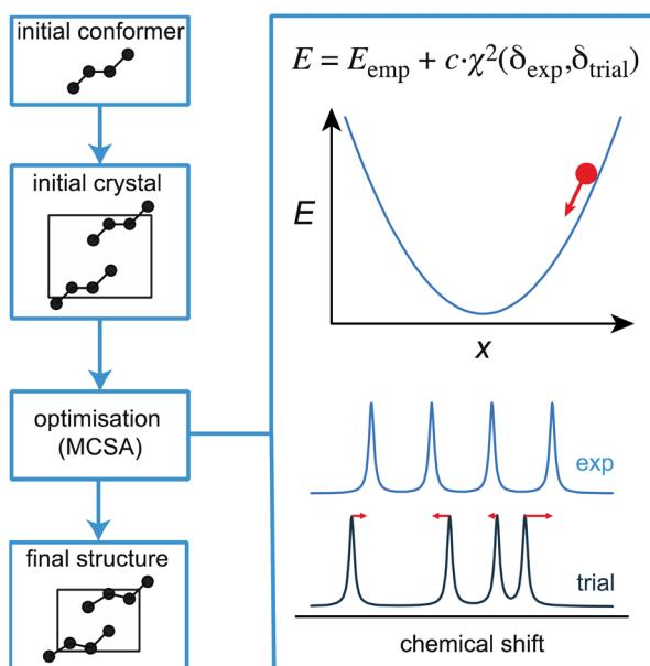
**Fig. 9** A schematic outline of one approach to direct structural optimisation using on-the-fly chemical shifts. The driving force for optimisation is an empirical energy term  $E$  that is the sum of a computed internal energy term  $E$  that ensures physically realistic structures, and a term that drives agreement between experimental and predicted chemical shifts.<sup>218</sup>
