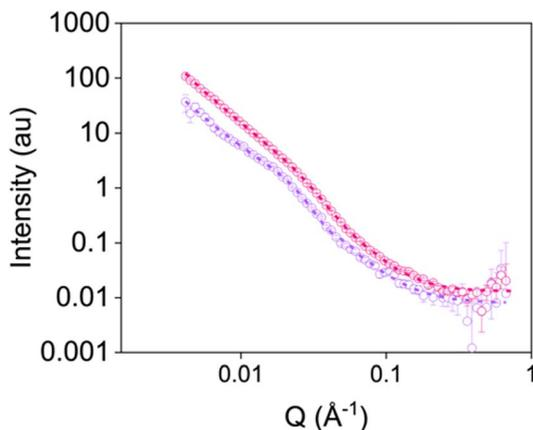
Fig. 6 Small-angle neutron scattering patterns for gels sheared at  $2500\text{ s}^{-1}$  using the rheometer (purple) and a syringe pump (pink). Open circles show the data and dashed lines represent the fit.
