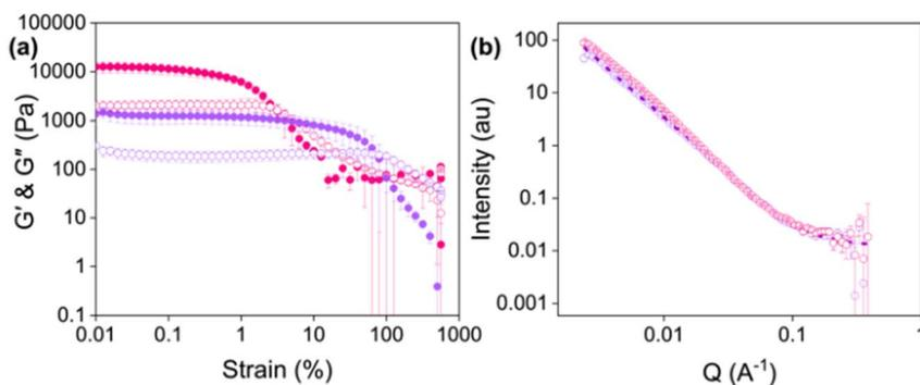
Fig. 4 (a) Strain sweeps of Gel-1 (purple) and Printed Gel-1 (pink). Closed circles represent  $G'$  and open circles represent  $G''$ . Data shown are averaged data for triplicate runs, with error bars representing standard deviation. (b) Small-angle neutron scattering patterns for Gel-1 (purple) and Printed Gel-1 (pink). Open circles show the data and dashed lines represent the fit.
