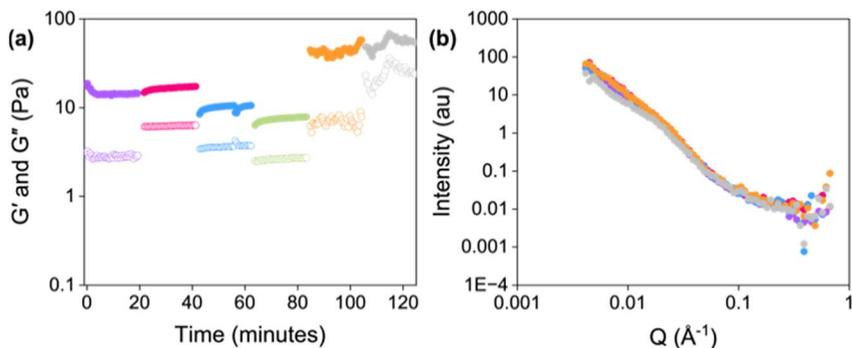
Fig. 5 (a) Change in  $G'$  and  $G''$  with increasing shear applied. Closed circles represent  $G'$  and open circles represent  $G''$ . (b) Small-angle neutron scattering patterns for Gel-1. Open circles show the data and dashed lines represent the fit. The gel was sheared at shear rates of 0 (purple), 1 (pink), 10 (blue), 100 (green), 1000 (orange), and 2500 (grey)  $\text{rad s}^{-1}$ .
