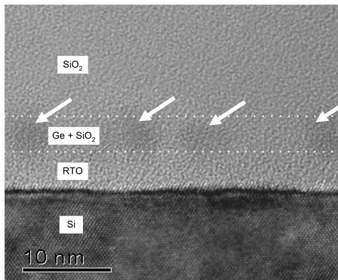
**Fig. 1** (a) Schematic diagram of the tri-layer insulator gate stack structure. (b) TEM cross-section showing the formation of germanium nanocrystals (indicated by white arrows) in a 3 nm thick middle layer (bound by dotted white lines) of the tri-layer insulator gate stack structure. (b) Reproduced with permission from ref. 70, Copyright 2002, AIP Publishing.
