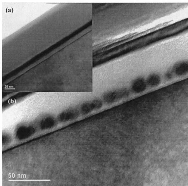
**Fig. 2** (a) Cross-section TEM micrograph of the  $\text{Si}_{0.54}\text{Ge}_{0.46}$  film that has been wet oxidized at 600 °C for 60 min. (b) Cross-section TEM micrograph of the Ge nanodots formed by annealing the structure shown in (a) in  $\text{N}_2$  for 300 s at 1000 °C. Reproduced with permission from ref. 74, Copyright 2004, AIP Publishing.
