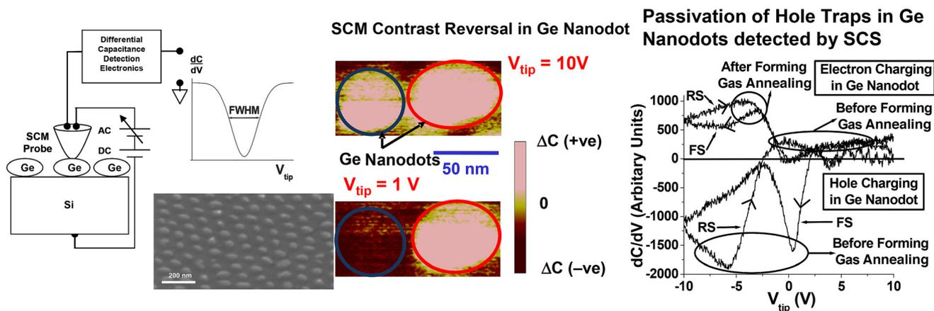
**Fig. 9** Scanning capacitance microscopy/microscopy (SCS/SCM) of Ge nanodots before and after forming gas annealing at 450 °C showing electron and hole charging in Ge nanodots. Reproduced with permission from ref. 75, Copyright 2008, AIP Publishing.
