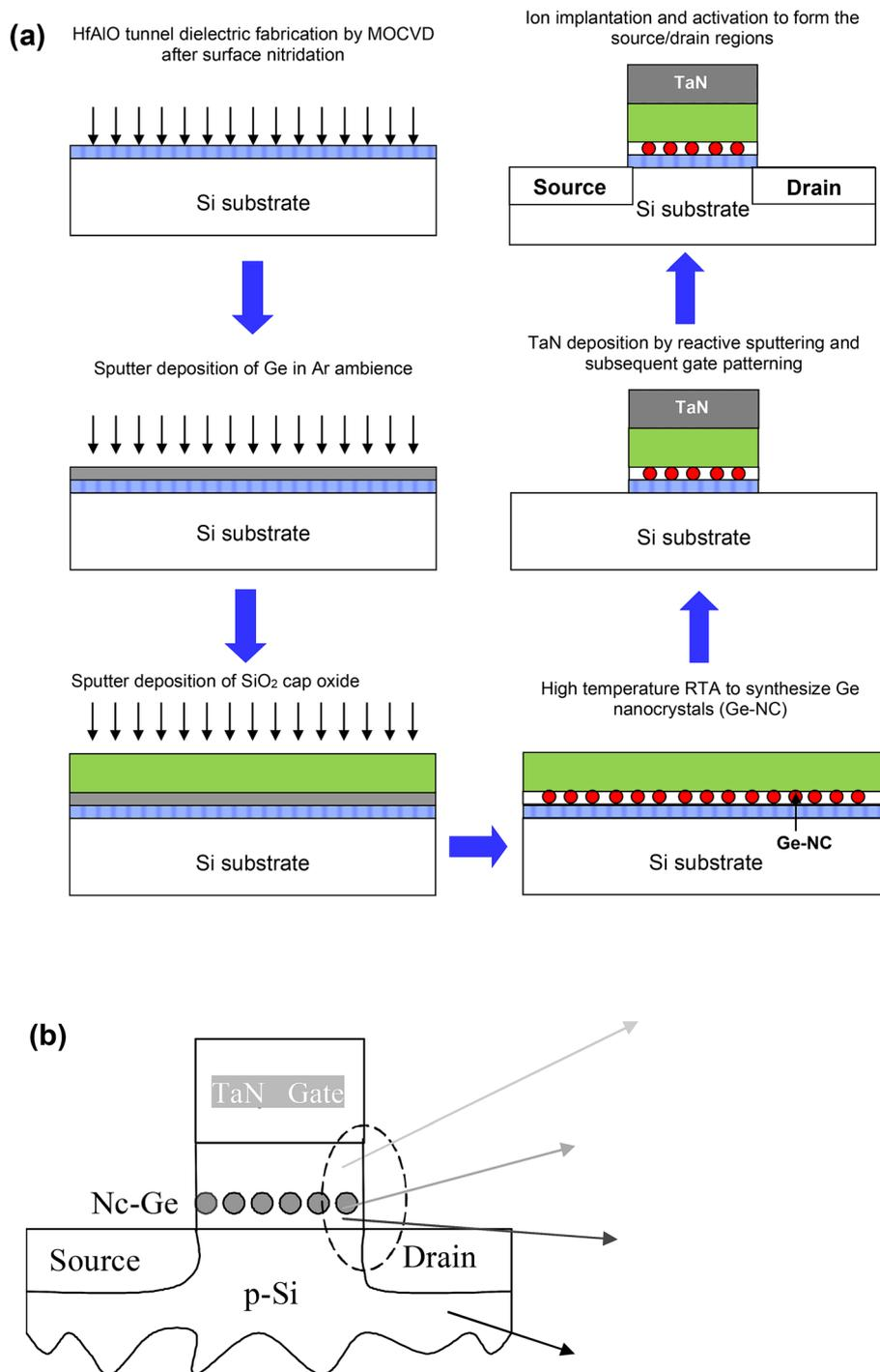
**Fig. 3** (a) Schematic diagram of the fabrication process flow of the Ge nanocrystal memory transistor. (b) Schematic and TEM cross-section of the Ge nanocrystal memory transistor showing the Ge nanocrystals formed in the middle layer of the tri-layer gate structure. (a) Reproduced with permission from ref. 73, Copyright 2023, American Chemical Society.
