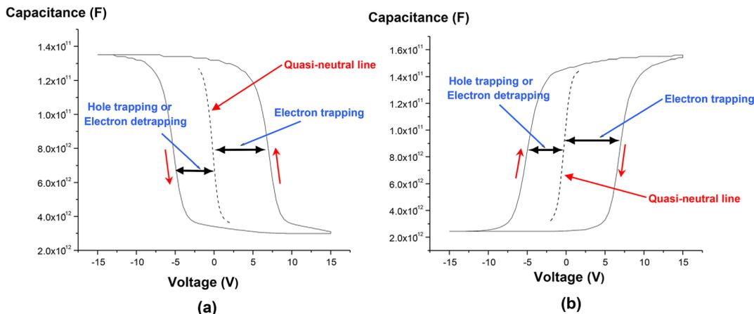
**Fig. 8** High-frequency C–V characteristics of capacitor tri-layer gate structures embedded with Ge nanocrystals and a silicon dioxide tunnel dielectric for (a) p-type and (b) n-type (100) Si substrates. Reproduced with permission from ref. 73, Copyright 2023, American Chemical Society.
