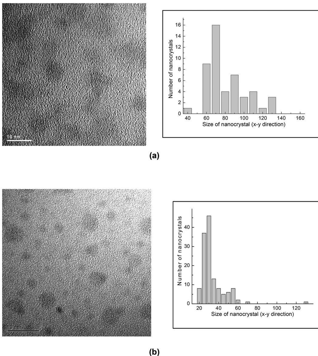
**Fig. 5** (a) Planar TEM image and size distribution histogram of the Ge nanocrystals of a trilayer structure consisting of 5 nm of tunnel oxide and 50 nm cap oxide with (a) a 6 nm thick middle layer (device D) and (b) a 3 nm thick middle layer (device E). Adapted with permission from ref. 70, Copyright 2002, AIP Publishing.
