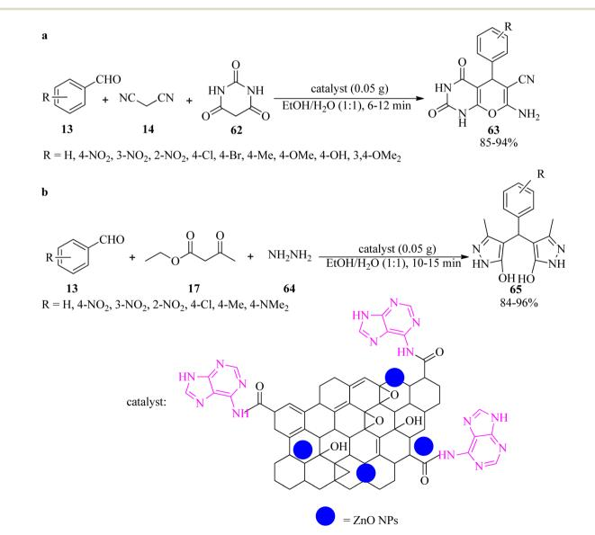
Scheme 20 Synthesis of (a) pyrano[2,3-d]pyrimidines, and (b) bis(pyrazol-5-ole) derivatives.
