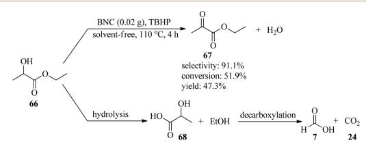
Scheme 21 Preparation of ethyl pyruvate (EP) from ethyl lactate (EL).
