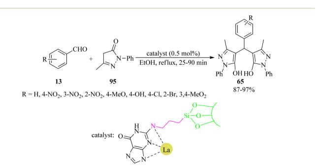
Scheme 29 Synthesis of 4,4'-(arylmethylene)-bis-(3-methyl-1-phenyl-1H-pyrazol-5-ol) derivatives.
