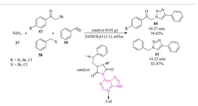
Scheme 19 Synthesis of 1,4-disubstitued 1,2,3-triazoles via click reaction.
