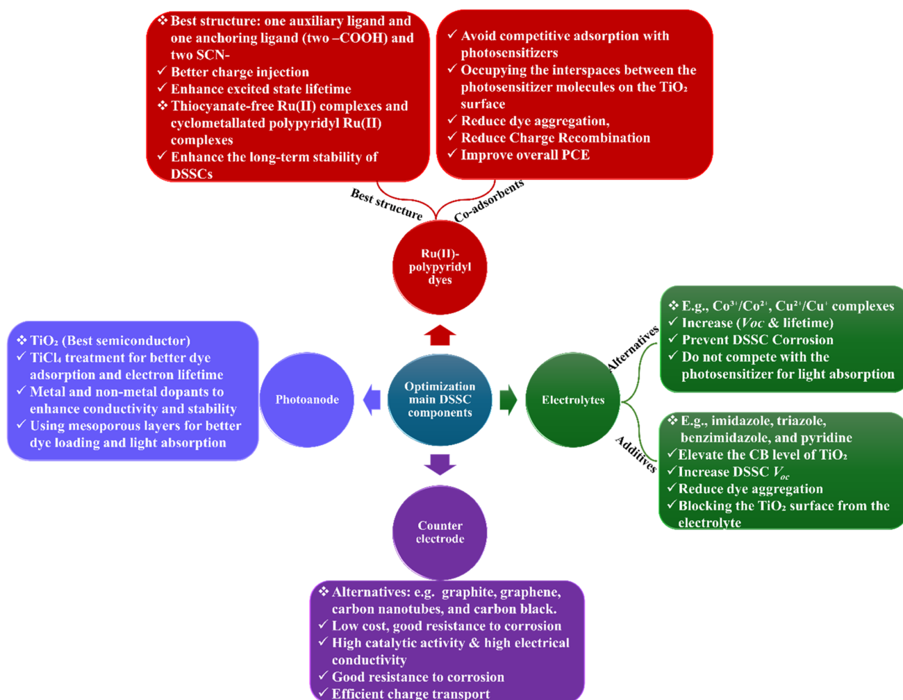
Fig. 1 The key optimization strategies of the DSSCs components including modifications to electrolytes, Ru(II)-polypyridyl dyes, co-adsorbents, counter electrodes, and additives.
