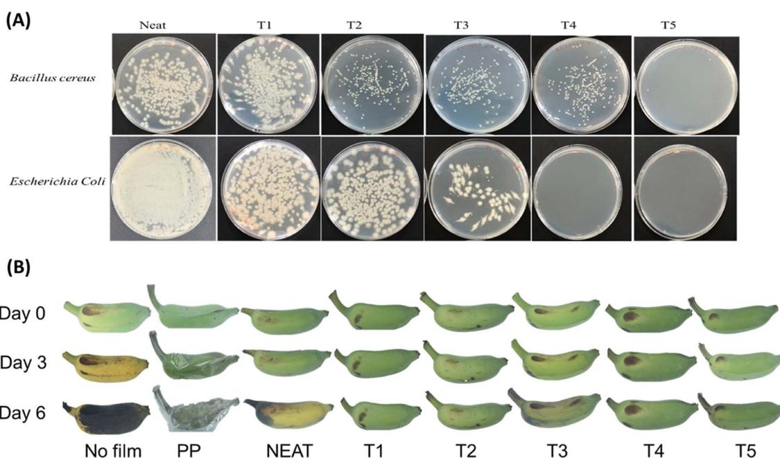
Fig. 12 (A) Antimicrobial effect of PBS/PBAT films with different  $\text{TiO}_2$  concentrations; and (B) comparison of the appearance of bananas in their natural state (no film) to those wrapped in PP and PBAT/PBS films with varying  $\text{TiO}_2$  levels [neat (0.9%), (T2) 1.8%, (T3) 2.7%, (T4) 3.6%, and (T5) 4.5%]. Reproduced with permission from ref. 201, Elsevier, 2023.
