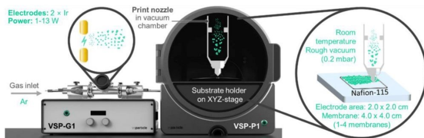
Figure 5. Schematic of the VSParticle nanoparticle printing technology. A certain wattage is applied to metal electrodes which causes the metal to ablate and particles to detach. The particles agglomerate to form nanoparticles as they are carried by inert Ar to a vacuum chamber where they are printed via nozzle onto a substrate of choice held by a XYZ-stage. Reproduced with permission from Reference 110. Copyright 2022 MDPI.
