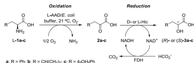
**Scheme 1** Redox cascade for the preparation of (*R*)- or (*S*)-hydroxy acids from L-amino acids.
