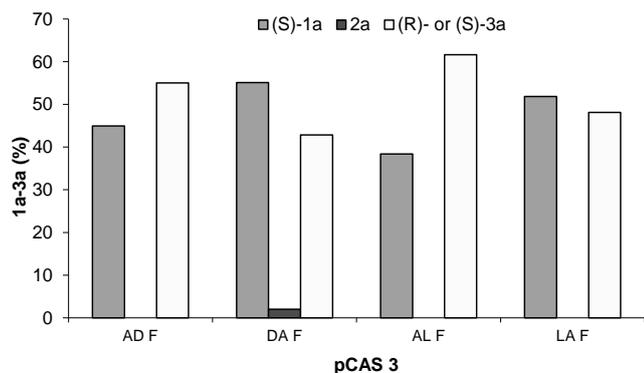
**Figure 2** Percentage of **1a-3a** after the transformation employing lyophilized *E. coli*/CAS3.1-4. Reaction conditions (*S*)-**1** 100 mM, O<sub>2</sub> 1 bar, *E. coli*/CAS3 (20 mg), NAD<sup>+</sup> (1 mM), HCO<sub>2</sub>NH<sub>4</sub> (300 mM), KP<sub>i</sub> (100 mM, pH 7), 1 h, 21 °C, 170 rpm.
