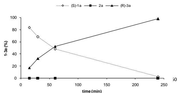
**Figure 4.** Time course of the transformation of L-**1a** employing lyophilized *E. coli*/pCAS3.1 cells. Reaction conditions (*S*)-**1a** 100 mM, O<sub>2</sub> 1 bar, *E. coli*/pCAS3.1 (20 mg), NAD<sup>+</sup> (1 mM), HCO<sub>2</sub>NH<sub>4</sub> (300 mM), KP<sub>i</sub> (100 mM, pH 7), 21 °C, 170 rpm.
