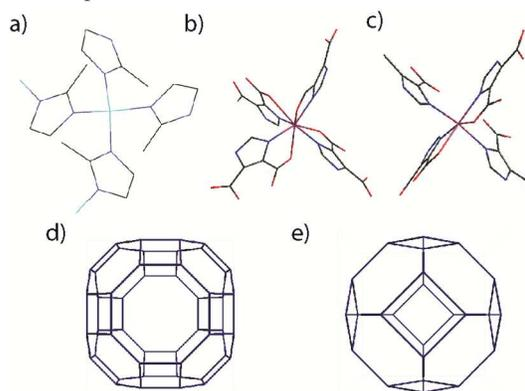
**Figure 1:** (a) Zn coordination environment in ZIF-8, (b) In 8-coordinate and (c) 6-coordinate environments in rho- and sod-ZMOF respectively. C – black, N – dark blue, O – red, In – pink, Zn – light blue, H atoms omitted. d) The ‘rho’ and (e) the ‘sod’ topologies/network architectures shared by ZIFs, ZMOFs and zeolites.
