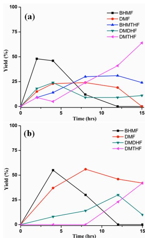
Figure 3. Time course of the Pd/C catalyzed reaction of HMF under H<sub>2</sub> (30 psi). (a): w/o acid. (b): CH<sub>3</sub>CO<sub>2</sub>H (10 equiv). Reaction conditions: substrate (0.5 mmol), substrate/Pd = 10 molar ratio, dioxane (5 mL), 120 °C.
