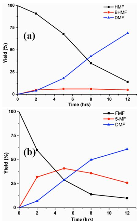
**Figure 1.** Time course of hydrogenolysis of HMF (a) and FMF (b) to DMF over time. Reaction conditions (see Scheme 2): 0.5 mmol substrate, substrate/Pd = 10 molar ratio, FA (10 equiv), dioxane (5 mL), 120 °C.
