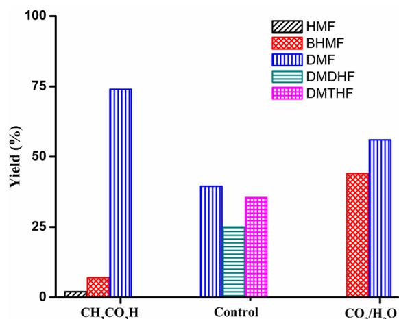
**Figure 5.** Product distribution for the reaction of HMF with Pd/C (substrate/Pd = 20 molar ratio). *Control:* no additive Reaction conditions: substrate (2 mmol), dioxane (5 mL), 120 °C, 15 h.
