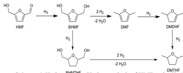
**Scheme 4.** Hydrogenation/Hydrogenolysis of HMF under H<sub>2</sub> (30 psi) with Pd/C.
