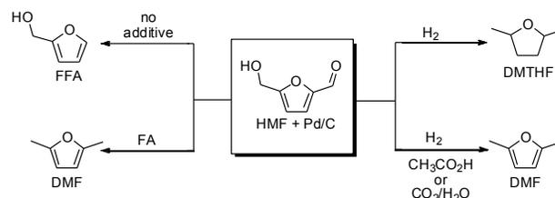
**Scheme 1.** Reaction of HMF catalyzed by Pd/C with and without additives. HMF: 5-hydroxymethylfurfural; FFA: furfuryl alcohol; DMF: dimethylfuran; FMF: 5-(formyloxymethyl)furfural; DMTHF: dimethyltetrahydrofuran.
