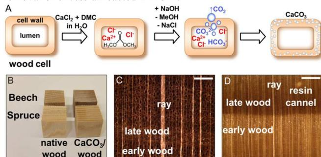
**Figure 1.** A: Schematic depiction of the mineralization of wood by alkaline hydrolysis of dimethyl carbonate in the presence of calcium ions within the wood matrix. B: Photo of unmodified and mineralised spruce and beech samples (2 cm edge length). Light microscopic images of mineralised beech (C) and spruce specimens (D). The scale bars in C and D correspond to 500  $\mu$ m.
