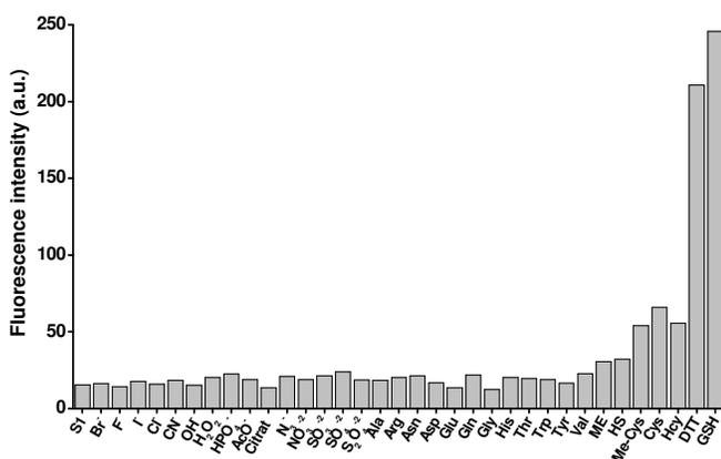
**Figure 4.** Emission intensity of safranin O at 575 nm (excitation at 520 nm) released from solid **S1** (water at pH 7.0) in the presence of selected anions, amino acids and reducing agents (10 mM) after 30 min upon addition.
