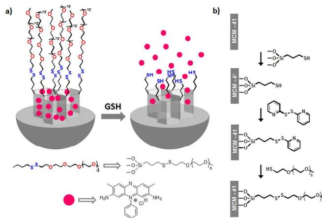
**Scheme 1.** (a) Schematic representation of the sensing mechanism of solid S1 in the presence of GSH. (b) Sequence of reactions used to anchor the molecular gate onto the outer surface of the loaded inorganic support.
