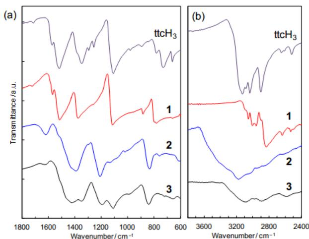
**Figure 4** FTIR spectra of **1**, **2** and **3** compared with pure trithiocyanuric acid. (a) 600–1800  $\text{cm}^{-1}$ . (b) 2400–3800  $\text{cm}^{-1}$ .
