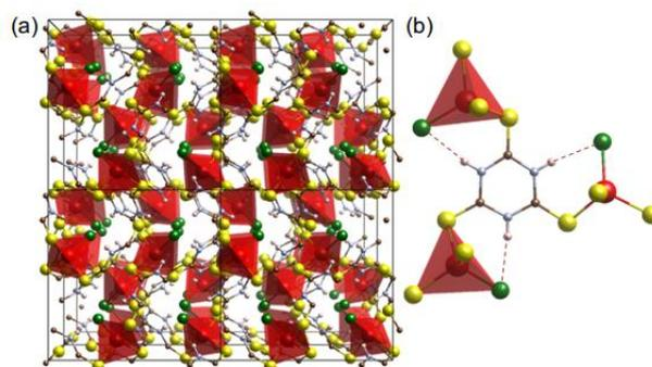
**Figure 1** Crystal structure of  $[\text{CuCl}(\text{ttcH}_3)]$ .<sup>13</sup> (a)  $2 \times 2 \times 2$  cells. (b) Connectivity of  $\text{CuClS}_3$  tetrahedral with the thioketone form of trithiocyanuric acid molecules (red: Cu, green: Cl, yellow: S, blue: N, brown: C, and white: H). Dotted lines show hydrogen bonding.
