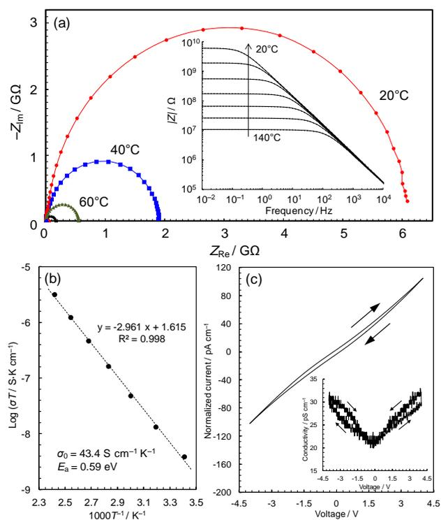
**Figure 3** AC Impedance analyses. (a) Complex-plane impedance data for a pellet of **3** (red: 20°C; blue: 40°C; green: 60°C; and black: 80°C). The inset shows  $\log |Z|$  vs  $\log$  frequency plots. (b) Arrhenius plot of the electronic conductivity. (c) Current-voltage characteristics measured by cyclic voltammetry scanned at 10  $\text{mV s}^{-1}$  at 25°C.
