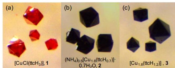
**Figure 2** Photos of (a) **1** CuCl(ttcH<sub>3</sub>) crystals, (b) **2** – *i.e.* **1** treated in aqueous ammonia for 2 days, and (c) **3** – *i.e.* **2** dried at 130°C under vacuum. The large monoliths are about 100  $\mu$ m across.
