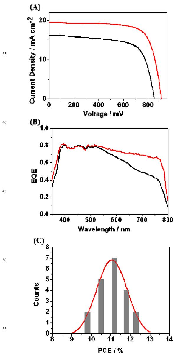
Fig.4  $I$ - $V$  curves (a) and  $EQE$  spectra (b) of the devices prepared the perovskite-coated TiO<sub>2</sub> films prepared at x=0 (black line) and 0.6 (red line), and histogram of PCEs for device 6 for 20 samples (c).
