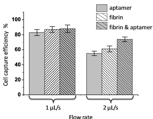
**Figure 4.** Cell capture comparison of aptamer alone, fibrin alone, and aptamer-fibrin combination. The capture efficiency was of  $10^3$ /mL CCRF-CEM cells in PBS buffer. Error bars represent one standard deviation ( $n = 3$ ).
