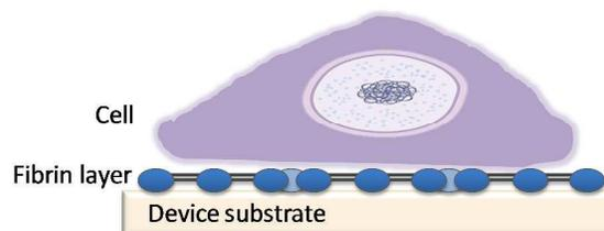
**Figure 1.** Schematic showing the fibrin-based tumor cell capture. The drawing is not to scale.
