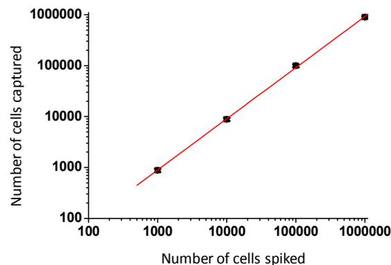
**Figure 3.** Calibration plot of cancer cell (CCRF-CEM cells) capture from PBS buffer solution with different cell concentrations at a flow rate of 1.0  $\mu\text{L/s}$ ; solid lines represent linear fitting. RSDs obtained from each the concentration are all below 10%.
