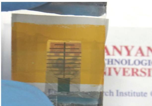
**Figure S8.** Photo of semi-transparent MAPbBr<sub>3</sub>/CNT solar cell with gold finger electrode.
