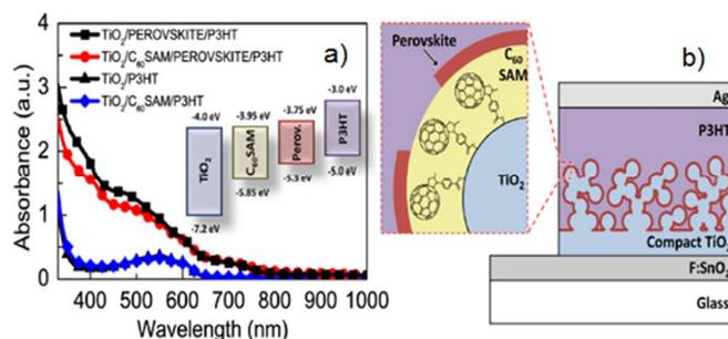
**Figure 7** – (a) UV-vis spectra of P<sub>3</sub>HT and perovskite films with and without C<sub>60</sub>SAM. Inset: the energy level of the components used in Snaith's work.<sup>85</sup> (b) The structure of the PSC fabricated with C<sub>60</sub>SAM layer between perovskite and TiO<sub>2</sub> layers. Reprinted with permission from ref. 85 © 2013, American Chemical Society.
