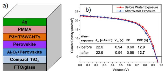
**Figure 6** – (a) Schematic illustration of PSC fabricated with CNTs/polymer composite as a hole collection layer as reported by Snaith's group.<sup>79</sup> (b) Current density–voltage curves of PSCs before and after water exposure for 60 sec (reprinted with permission from ref. 79 © 2014, American Chemical Society).
