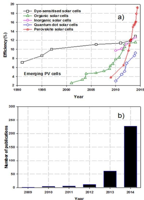
**Figure 1** – (a) Efficiency records vs. Year of third generation (emerging) PVs. The red line indicates that the efficiency of PSCs has improved dramatically in the past 2 years. (b) Number of publications (since 2009) that appeared in Scopus on 28<sup>th</sup> September, 2014. Keyword used in the search was “Perovskite Solar Cells” in the title of the article.
