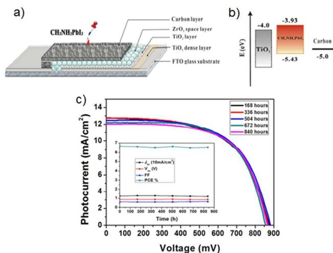
**Figure 4** – (a) The structure of the first carbon counter electrode based PSC.<sup>64</sup> (b) Energy level of TiO<sub>2</sub>, CH<sub>3</sub>NH<sub>3</sub>PbI<sub>3</sub> and carbon.<sup>64</sup> (c) Current density–voltage curves of carbon cathode based PSCs over 840 hours. Inset: the effect of time on each value ( $J_{sc}$ ,  $V_{oc}$ , FF and PCE) of solar cell. Reprinted with permission from ref. 64 © 2013, Nature Publishing Group.
