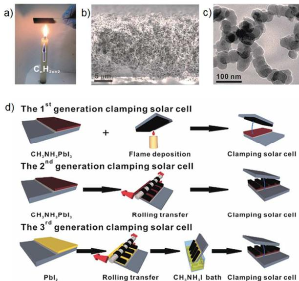
**Figure 5** – (a) Digital photo of the candle-soot film preparation. (b) Cross sectional SEM image of the candle-soot film. (c) TEM image of the as-prepared candle-soot particles. (d) Fabrication processes of the candle-soot film based PSCs. Reprinted from ref. 70.
