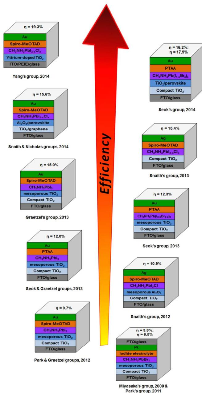
**Figure 3** – Progress in the efficiency record of PSCs since 2009 showing the structures of PSCs (constructed by the corresponding groups) used to achieve the reported energy conversion efficiencies. These PSCs have been reported in references 13-24.<sup>13-24</sup>
