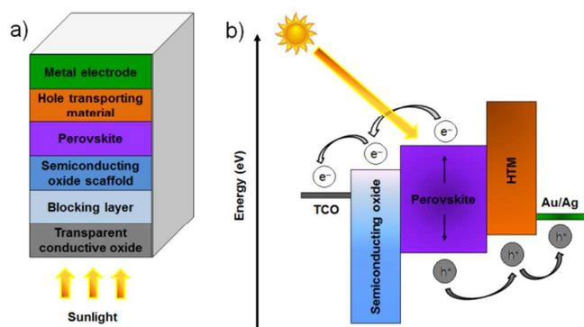
**Figure 2** – (a) Structure and (b) operational mechanism of a typical PSC.
