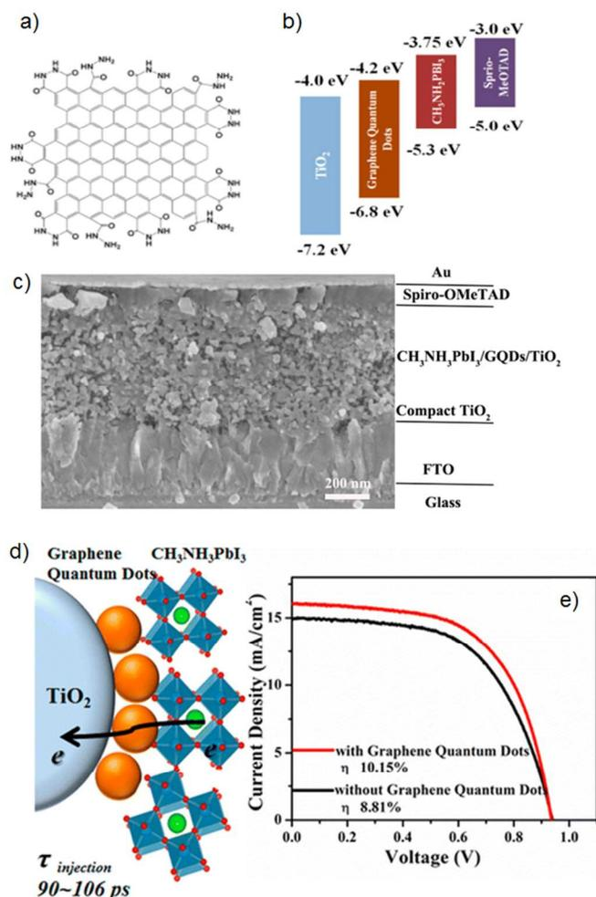
**Figure 8** – (a) Schematic of GQD structure. (b) Energy levels of different layers used in PSCs of Zhu et al.<sup>81</sup>, (c) Cross sectional SEM image of PSCs fabricated with GQDs. (d) Schematic illustration of electron generation and injection at the interfaces of TiO<sub>2</sub>, GQDs and perovskites. (e) Current density–voltage curves for the best performing PSCs. Reprinted with permission from ref. 81 © 2014, American Chemical Society.
