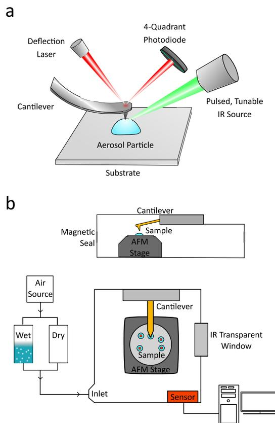
**Fig. 1** a) An illustrative representation of the main AFM-PTIR components is shown in the overhead configuration. b) Schematic of the environmental chamber used for relative humidity studies: top panel-side view, and bottom panel-top view.
