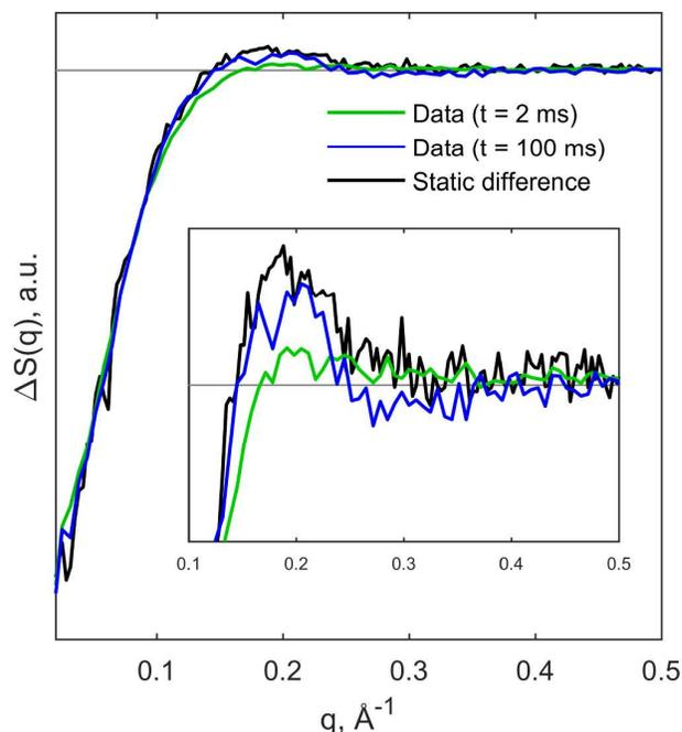
Figure 3. Comparison of the protein associated TRXSS data recorded at 2ms and 100 ms time delays with reference difference data calculated from static SAXS curves collected at 20 and 15  $^\circ\text{C}$ .
