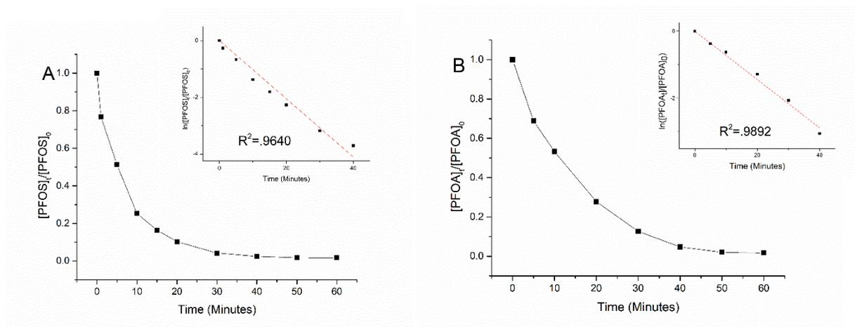
**Figure 1.** The concentration of PFOS (A) and PFOA (B) over time during electrooxidation with TSO anode at  $5.0 \text{ mA}\cdot\text{cm}^{-2}$ . The test solutions contained each PFAA individually at the Initial concentration of  $2.0 \text{ }\mu\text{M}$  in  $100 \text{ mM Na}_2\text{SO}_4$  as supporting electrolyte. Insert shows fit to the pseudo-first rate model.
