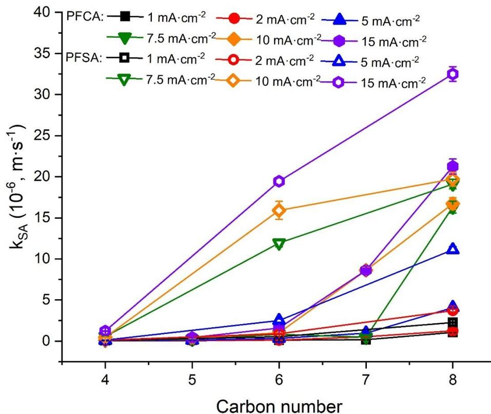
**Figure 3.** The  $k_{SA}$  values of PFAAs of different carbon chain lengths and head functional groups, obtained in electrooxidation experiment with TSO anodes at different current densities. The test solutions contained all PFAAs in mixture with each at the initial solution of was 2.0  $\mu\text{M}$  in 100-mM  $\text{Na}_2\text{SO}_4$  as supporting electrolyte. Error bar represents standard deviation.
