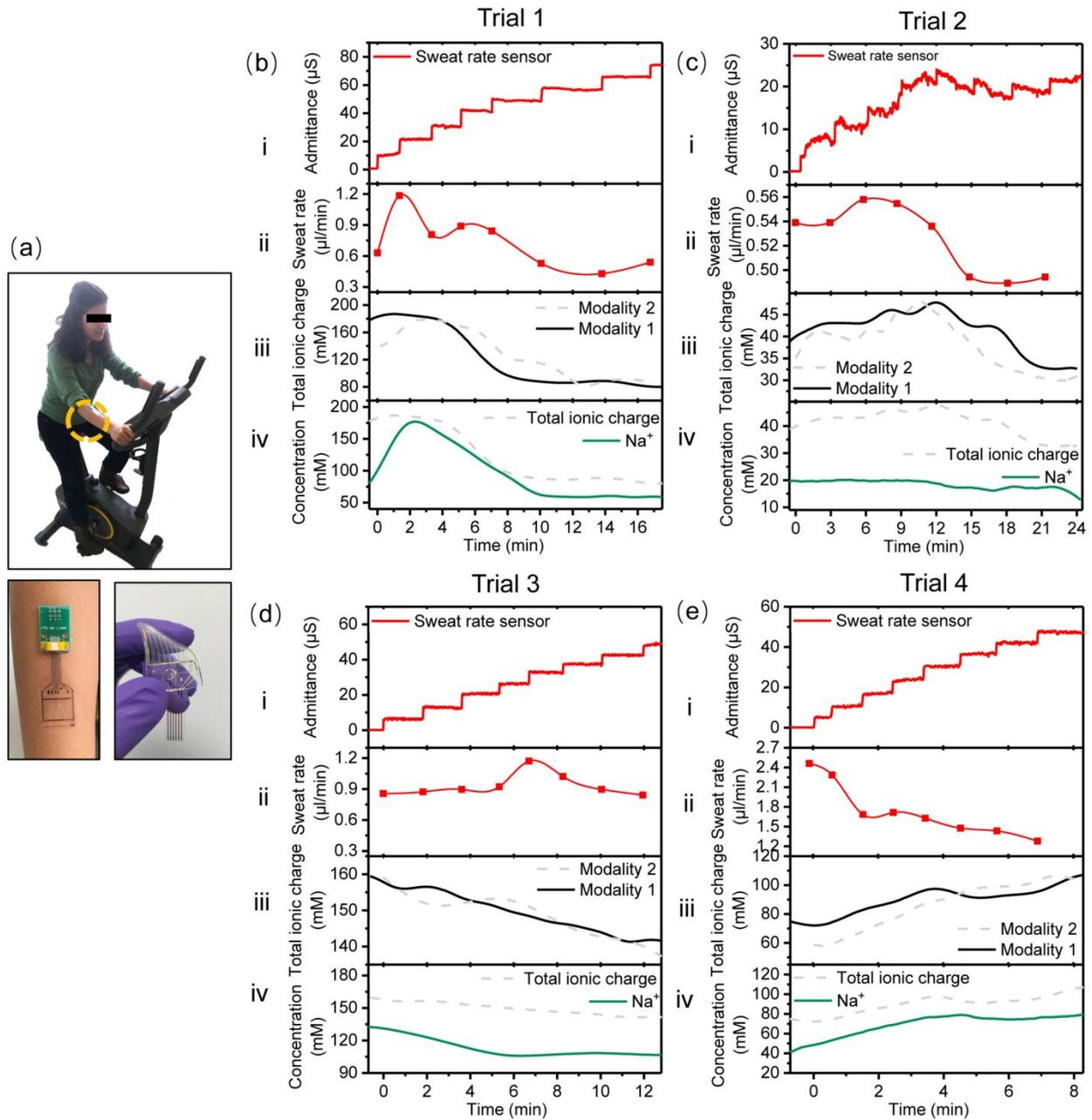
**Fig. 6.** Real-time, on-body sweat analysis during stationary biking exercise. (a) Optical image of subject with multi-modal sweat sensing patch affixed to their forearm, with connector board for signal read-out. (b)-(e) On-body sweat analysis Trials 1-4 respectively, showing simultaneous measurement of (i) raw sweat rate sensor
