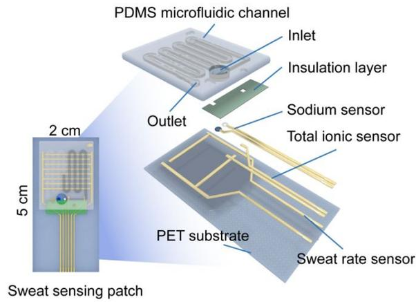
**Fig. 1.** Schematic of multi-modal sweat sensing patch with sensors for sweat rate, total ionic charge concentration, and  $\text{Na}^+$  ion concentration located within a PDMS microfluidic for sweat capture and flow.
