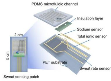
A wearable, multi-modal sensing patch for sweat rate and electrolyte analysis with inbuilt cross-verification schemes to ensure data integrity.
