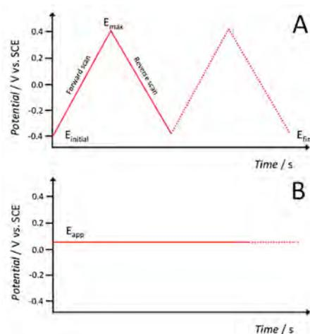
Figure 3. Cyclic voltammetry triangular potential waveform (A) for a scan between -0.4 and +0.4 V vs. SCE. Constant potential applied in amperometric i-t curves (B).
