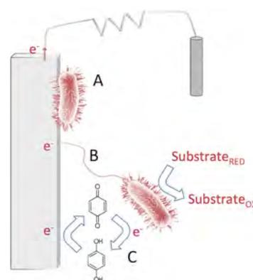
Figure 1. Scheme of the three extracellular electron transfer pathways in bioelectrochemical systems with intact bacterial cells as the biological catalyst for substrate oxidation. Direct extracellular electron transfer through membrane bound
