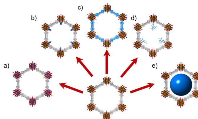
**Figure 2.** Post-synthetic modification scheme exhibiting a) cation exchange of node-based metals, b) condensed- or vapor-phase deposition of metal ions/clusters at the node, c) solvent assisted linker exchange (SALE) of structural ligands, d) solvent assisted ligand incorporation (SALI) of non-structural ligands, and e) encapsulation of catalytic species, such as nanoparticles, within the pores.
