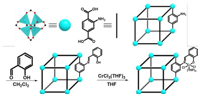
**Figure 4.** Zn node (top-left) and terephthalate linker (top-middle) of IRMOF-3 (top-right). Post-synthetic modification scheme of IRMOF-3-SI-Cr (bottom). Atom colours: Zn (light blue), O (red), C (black).
