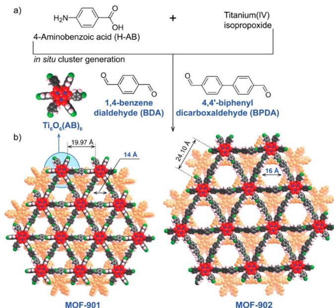
**Figure 11.** a) Synthesis procedure and b) crystal structures of MOF-901 and MOF-902. Atom colours: Ti (blue), C (black), O (red), N (green), H (pink), and second layer (orange). Reprinted with permission.<sup>54</sup> Copyright 2017 American Chemical Society.
