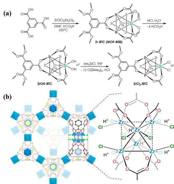
**Figure 7.** a)  $ZrCl_2$ -BTC synthetic scheme beginning with synthesis of Zr-BTC (MOF-808) and b) proposed structure of  $ZrCl_2$ -BTC. Reprinted with permission.<sup>41</sup> Copyright 2017 American Chemical Society.
