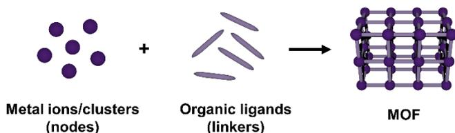
**Figure 3.** Schematic of the general formation of MOFs through assembly of inorganic (nodes) and organic (linkers) building units into a 3D structure.
