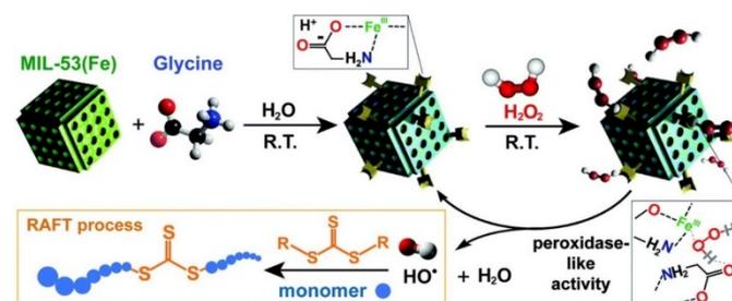
**Figure 10.** Proposed mechanisms for the formation of Gly/MIL-53(Fe) and the initiation of RAFT polymerization by hydroxyl radicals. Reproduced with permission.<sup>51</sup> Copyright 2018 The Royal Society of Chemistry.
