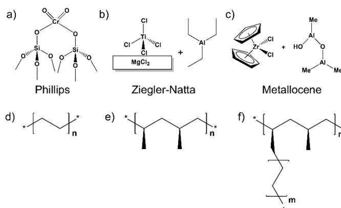
**Figure 1.** Structures of a) Phillips catalyst (proposed), b) Ziegler-Natta supported catalyst, c) example metallocene catalyst, d) linear polyethylene, e) isotactic polypropylene, and f) example specialty copolymer of propylene and ethylene.
