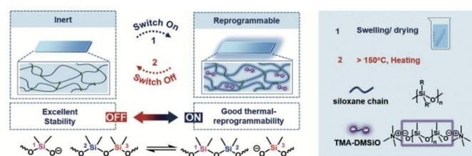
Figure 8. The schematic illustration of an LCE with siloxane bonds. Reproduced with permission from Ref.84. Copyright 2020, John Wiley and Sons.
