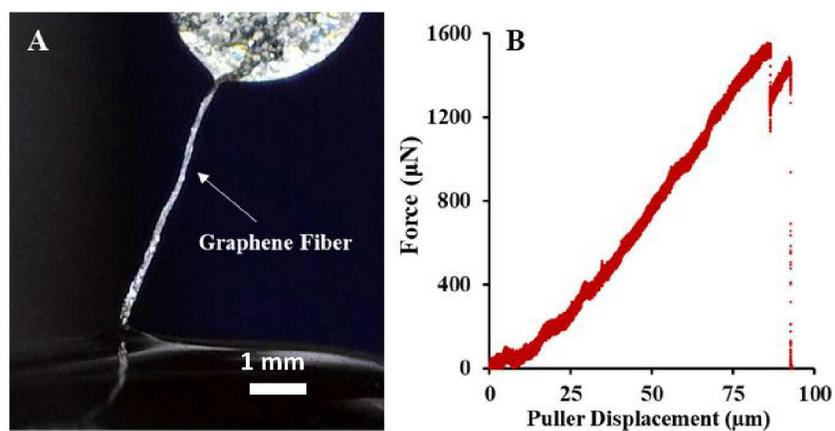
**Figure 3. Macroscale graphene fiber tested in uniaxial tension.** A, optical image of graphene fiber ( $A_{\text{graphene}} = 3.18 \mu\text{m}^2$ ,  $L_{\text{fiber}} = 2952 \mu\text{m}$ ). B, Force-displacement plot of uniaxial tensile test (puller displacement rate  $r_p = 0.50 \mu\text{m/s}$ ). This fiber exhibited brittle fracture, with a tensile strength of 0.475 GPa.
