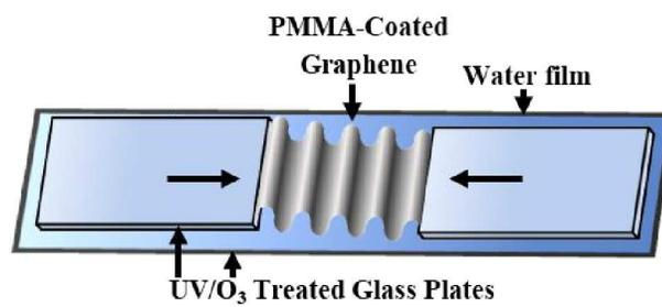
**Figure 1.** Schematic of folding process for PMMA-coated graphene in an accordion-like pattern. Glass plates were treated with  $UV/O_3$  prior to use. Wrinkles formed in the graphene sheet during compression along the width of the graphene sheet and remained folded as the sheet was compressed further.
