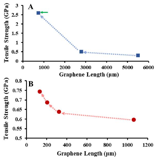
**Figure 5. Breaking strength of graphene fibers as a function of fiber length.** Dotted arrows indicate order of sequential uniaxial tensile tests on the same fibers with  $A_{\text{graphene}} = 3.2 \mu\text{m}^2$  (A) and  $A_{\text{graphene}} = 5.2 \mu\text{m}^2$ . (B). Green arrow indicates a measurement where ductile fracture behavior was observed during tensile testing.
