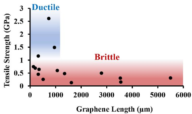
**Figure 6. Breaking strength of parent and fragment fibers.** Three fiber fragments exhibited ductile behavior and exhibited the largest measured breaking strengths. Brittle fracturing behavior was observed for most fibers.
