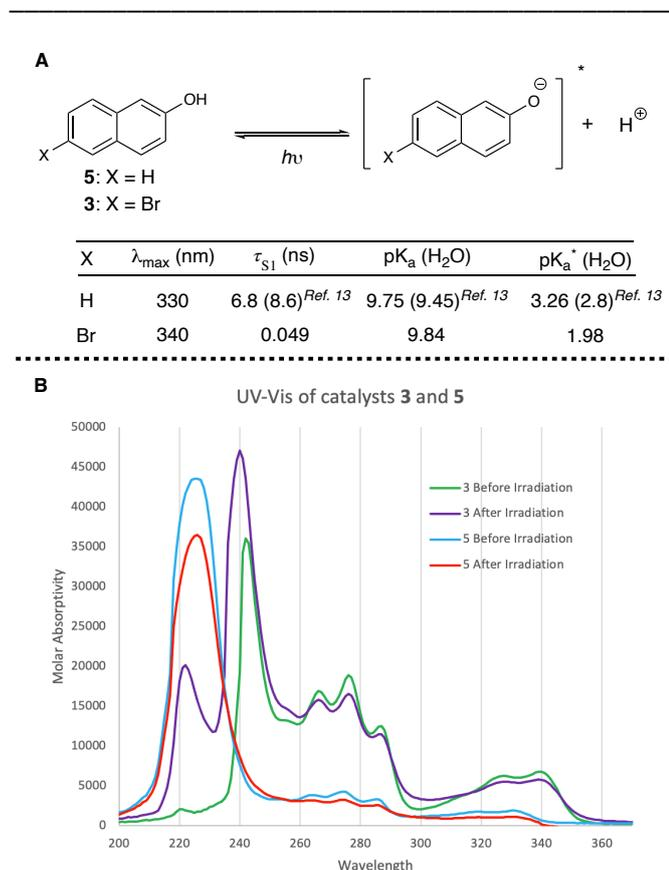
A) Excited-state  $pK_a$  and lifetime determination for catalysts **3** and **5**. B) UV-vis spectra for **3** and **5** before and after 18 h irradiation with Blue LEDs (5 mM in MeOH).
