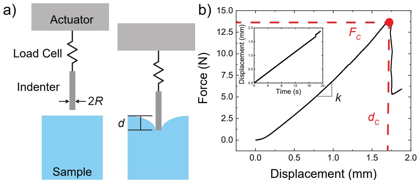
**Fig. 2** a) Sketch of the deep indentation and puncture measurements. b) Plot of the force displacement curve with the critical puncture force and displacement marked in red. The inset graph shows the displacement vs time profile.
