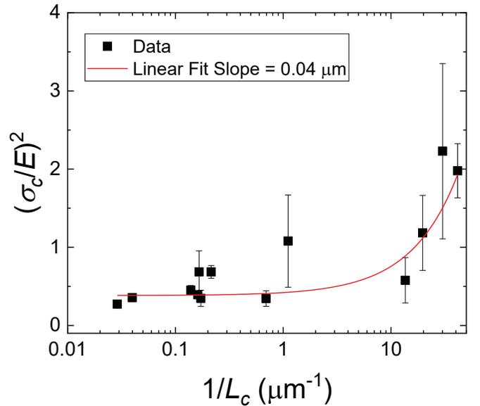
**Fig. 5** Plot showing  $(\sigma_c/E)^2$  against  $1/L_c$  for the composite hydrogels used in this study. Note that the x-axis is plotted in log scale. The slope on this plot,  $0.04 \mu\text{m}$ , is well below the elastofracture length of these materials and no significant transition is observed. This likely indicates that the assumption that  $a = L_c$  in the absence of a macroscopic notch is incorrect.
