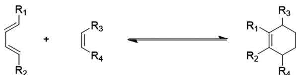
Scheme 4 Bond formation resulting from the Diels–Alder reaction and retro-Diels–Alder reaction.
