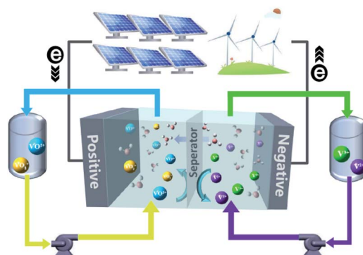
Fig. 1 A schematic diagram of a VFB.
