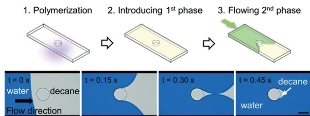
**Fig. 3** Single post oil–water displacement experiments. After building a single post in a microchannel and rinsing the channel with acetone to remove any uncured precursor solution, two immiscible fluids were serially introduced into the channel (decane followed by water). Scale bar is 100  $\mu\text{m}$ .
