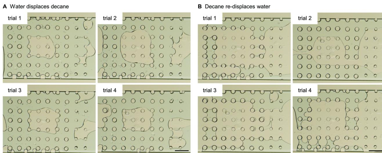
**Fig. 8** For the same multi-post microfluidic channel used in Fig. 7, we repeated the same decane/water displacement experiments, and counted how many posts held the displaced phase after the other phase was introduced. Images after (A) water displaces decane, and (B) decane re-displaces water. Scale bar is 200  $\mu\text{m}$ .
