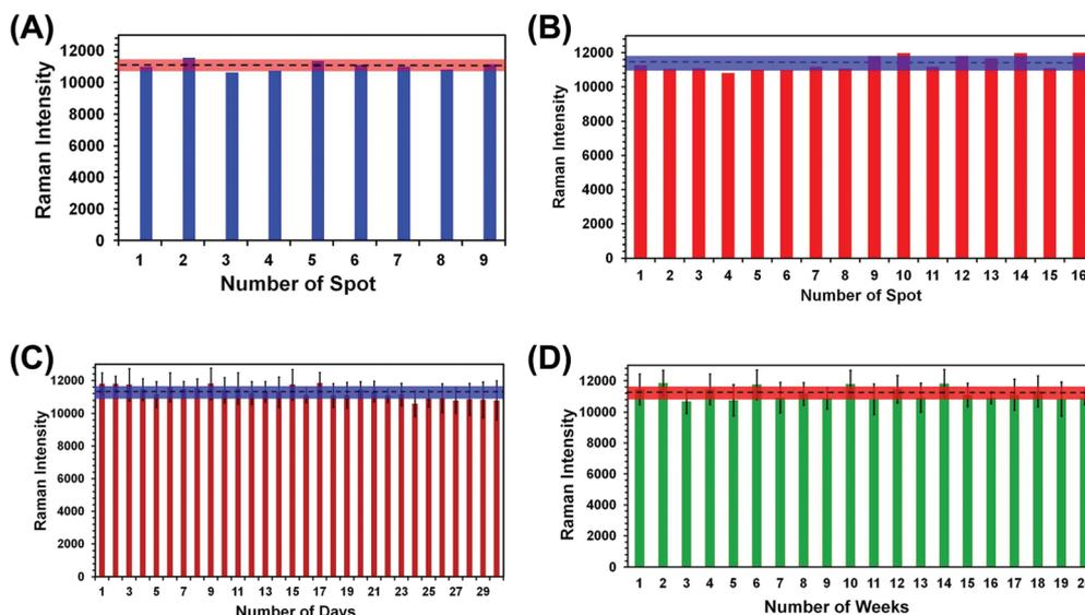
Fig. 4 Histograms of SERS intensity of TNT at 1380  $\text{cm}^{-1}$  collected from (A) 9 randomly selected spots on a particular nanosensor; (B) four randomly selected areas of four different nanosensors (1–4, 5–8, 9–12, and 13–16), which were prepared from four different batches of Au TNPs; (C) one SERS nanosensor over an entire month; (D) 20 individual nanosensors over the course of 5 months. The error bars in (C) and (D) represent measurements from six spots each.
