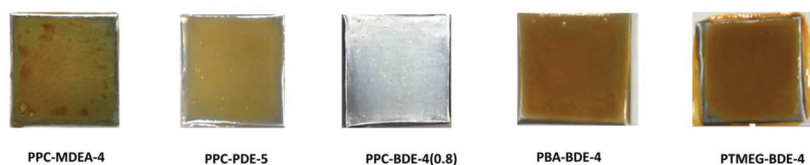
Fig. 3 Photographs of CS plates coated with PPC-MDEA-4 (far left), PPC-PDE-5 (left), PPC-BDE-4(0.8) (middle), PBA-BDE-4 (right) and PTMEG-BDE-4 (far right).
