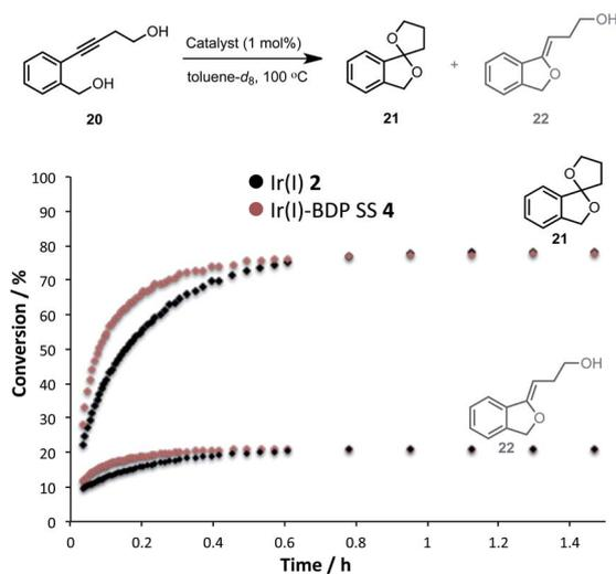
Fig. 10 Formation of the products **21** and **22** over time, monitored using *in situ*  $^1\text{H}$  NMR spectroscopy. Conditions: diol **20** (0.2 mmol), catalyst (0.002 mmol), toluene- $d_8$  (0.5 mL) under argon. Conversion calculated relative to the starting material **20**.
