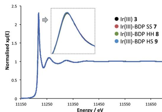
Fig. 9 The XAS spectra at the Ir L<sub>3</sub> edge for the Ir(III) based complexes.
