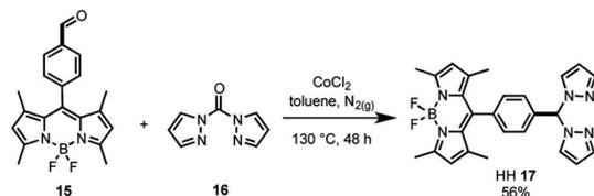
Scheme 2 Synthesis of the bifunctional catalyst framework HH 17.
