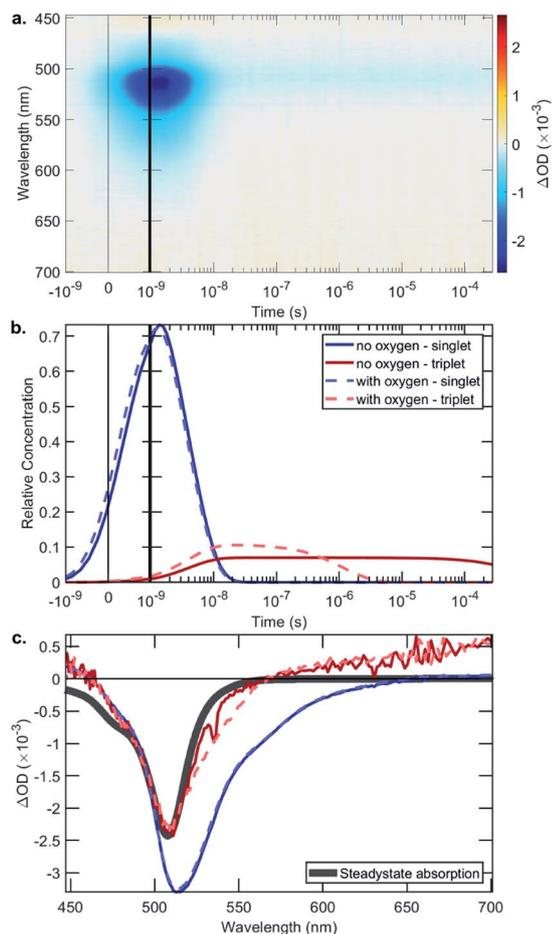
Fig. 6 The data from the transient absorption spectroscopy measurements for Ir(I)-BDP SS 4, chosen as a representative example: (a) the collected data, in the absence of oxygen, using an excitation wavelength of 355 nm; (b) fitted exponential decay showing the time dependent behaviour of the singlet and triplet excited states; and (c) the species associated spectra.
