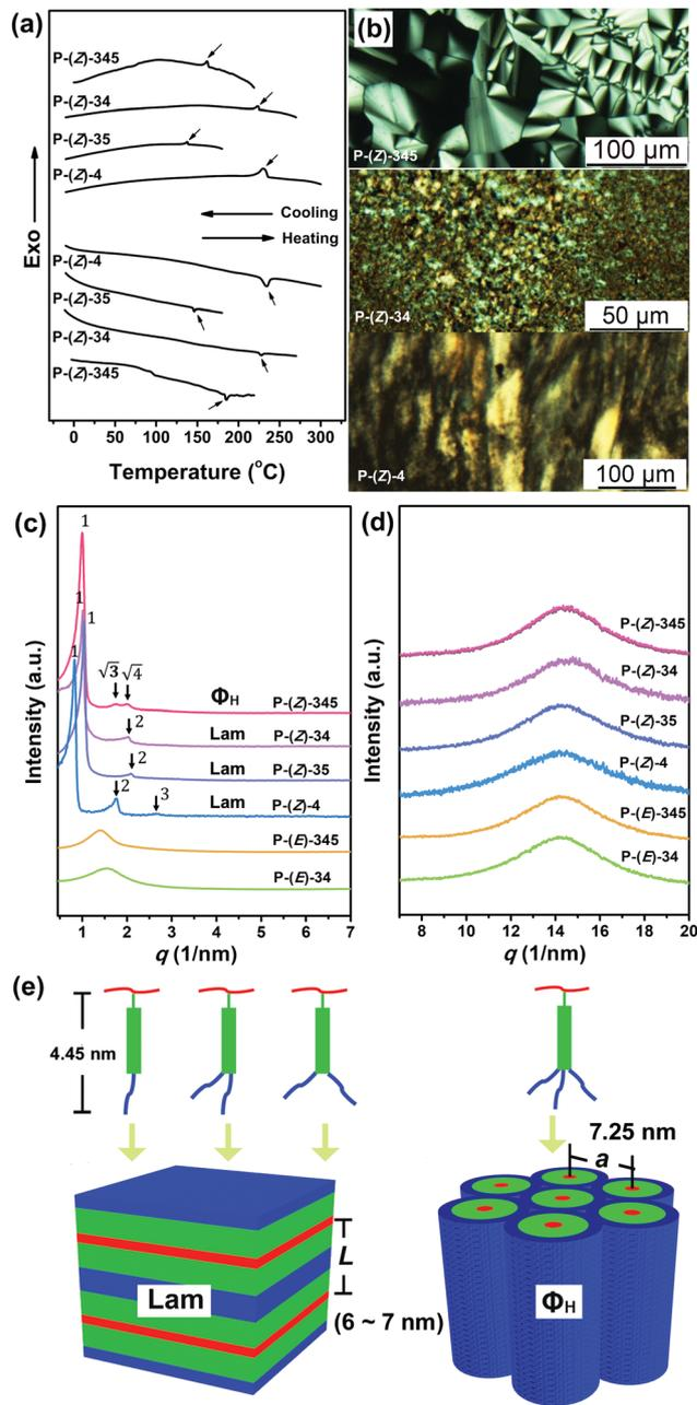
**Fig. 3** (a) DSC curves of polymers at a heating and cooling rate of 10 °C min<sup>-1</sup>. (b) POM pictures of P-(Z)-345 at 150 °C, P-(Z)-34 at 201 °C and P-(Z)-4 at 210 °C. SAXS (c) and WAXS (d) profiles of thermally annealed polymers recorded at room temperature. (e) schematic illustration of the phase structure model of smectic and  $\Phi_H$  phases.
