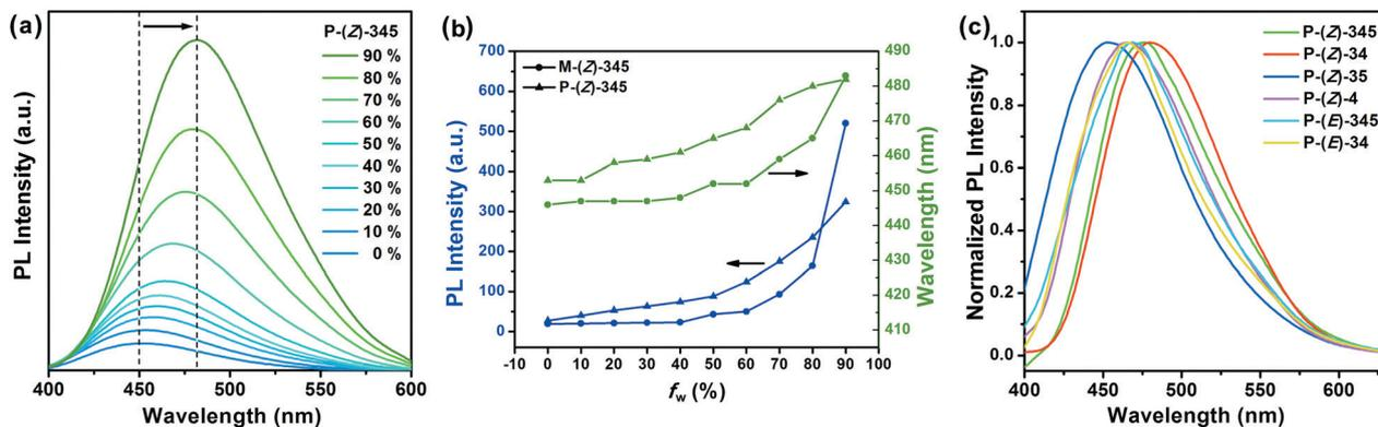
Fig. 5 (a) PL spectral changes of P-(Z)-345 depending on the water fractions in THF. (b) PL intensity and wavelength of M-(Z)-345 and P-(Z)-345 as a function of water content ( $f_w$ ) in THF/water mixtures. (c) PL spectra of polymer films.
