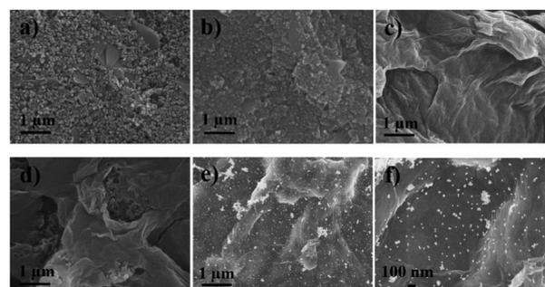
Fig. 2 SEM images of (a) SPCE, (b) GQDs/SPCE, (c) GO/SPCE, (d) GQDs/GO/SPCE, and AuNPs/GQDs/GO/SPCE with (e) low magnification ( $\times 20\,000$ ) and (f) high magnification ( $\times 50\,000$ ). The bright spots or small particles in (e) and (f) are AuNPs.
