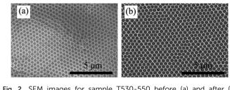
Fig. 2 SEM images for sample T530-550 before (a) and after (b) aqueous immersion.
