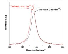
Fig. 3 Raman spectra of samples T530-550 and T530-550 in illustrating the shift of the main  $E_g$  peak from the presence of sulphur ions.
