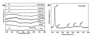
Fig. 1 Raman spectra of: (a) TiOSO<sub>4</sub> (TOS) and of TiO<sub>2</sub> IOs templated from 530 nm diameter PS spheres and calcined at different temperatures, including sample T530-550 after immersion; (b) Raman spectrum of sample T530-550im alone, exhibiting the peaks of anatase TiO<sub>2</sub>.
