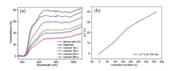
**Fig. 8** (a) Transmittance spectra of the EC device in the as prepared state (solid black line); colored at 3.5 V for 90 s (pink downward triangle), 180 s (green left triangle), 240 s (dark blue, right triangle) and 360 s (red cross); and bleached at -3.5 V for 360 s (blue triangle); (b) changes of optical contrast at visible range (700 nm) with coloration duration.
