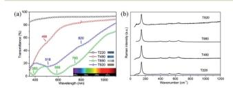
Fig. 7 (a) UV-vis-NIR transmittance spectra for samples T220 (black squares), T480 (red circles), T880 (green up-triangles) and T920 (blue left-triangles); (b) Raman spectra of the corresponding 2D  $TiO_2$  IO films. Inset in (a) show the film's optical reflection images.
