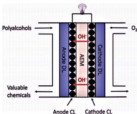
Fig. 4 Schematic diagram of the Anion Exchange Membrane Fuel Cell. Reproduced from ref. 44, Copyright 2017, Elsevier [CL = catalyst layer, DL = diffusion layer, AEM = anion exchange membrane].
