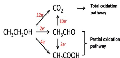
Fig. 2 Schematic diagram of the parallel pathways during the ethanol oxidation reaction. Reproduced from ref. 13, Copyright 2005, Elsevier.
