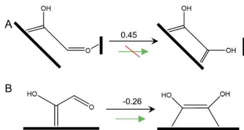
Scheme 1 Tautomerization of  $*\text{COH-CHO}$  on (A) Cu-DAN surface and (B) planar Cu(100). The values shown above arrows are  $\Delta G$  (eV) at 0 V vs. RHE.
