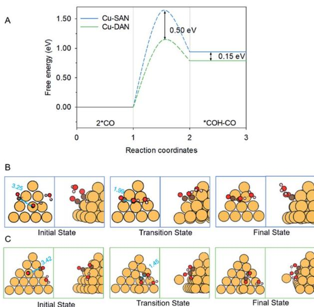
Fig. 3 (A) Reaction energetics involved in 2 \*CO dimerization and reduction to \*COH-CO at 0 V vs. RHE. Structures of the initial, transition and final states in CO-CO coupling on (B) Cu-SAN and (C) Cu-DAN, respectively. Minimum energy path for reaction barriers in panel A is found in Fig. S3.<sup>†</sup> Color code: Cu, orange; C, brown; O, red; H, pink. Distances are in Å.
