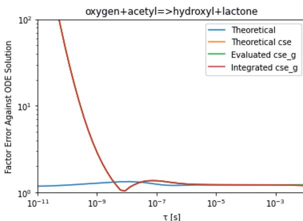
Fig. 11 Factor error in the flux from oxygen + acetyl in the decay case to hydroxyl + lactone at 0.01 bar and 500 K for  $t = \tau$  between a benchmark ODE solution of eqn (17) and the theoretical solution from eqn (33), theoretical cse from eqn (34), cse\_g evaluated at the benchmark, and integrated cse.
