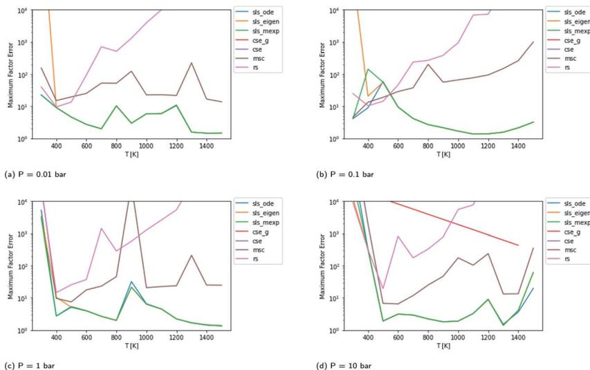
Fig. 4 Scores for each method at different pressures and temperatures for the acetyl + O<sub>2</sub> case study with the isomerization barrier lowered by 20 kcal mol<sup>-1</sup>. The CSE methods fail at most conditions in this case. The SLS methods overlap at high temperatures, with sls\_eigen diverging at low temperatures.
