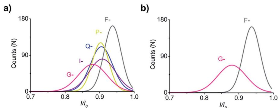
Fig. 8 Identification of the randomly selected five amino acids (I, F, G, P, and Q) using the negatively charged bipolar peptide probe  $D_6XR_5$ . (a) Histograms of  $I/I_0$  values of I-, F-, G-, P-, and Q-. (b) Histograms of  $I/I_0$  values of F- and G-.
