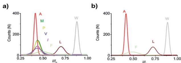
Fig. 3 Superimposed  $I/I_0$  histograms of A, V, L, P, W, M, and F (a).  $I/I_0$  histograms of A, F, L, and W (b). For each histogram, at least 1000 events were analysed, and the same applies to the figures below.
