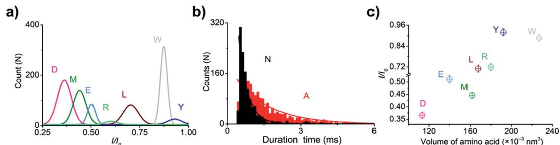
Fig. 7 Identification of proteinogenic amino acids via an aerolysin nanopore with the bipolar peptide probe  $D_4XR_5$ . (a) Identification of D, M, E, R, L, W, and Y based on the  $I/I_0$  values. (b) Comparison of the duration times of A and N at +70 mV. (c) Relationship of current amplitude against volume of the seven amino acids.
