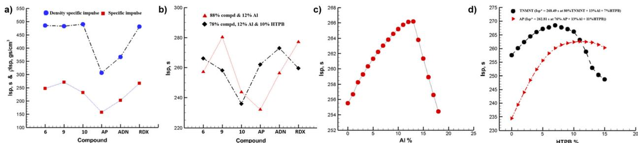
Fig. 3 (a) Comparison of propulsive properties (a) monopropellant (b) composite bipropellant. (c) **TMNMT** at 10% HTPB and varying the percentage of **TMNMT** (90–72%) and **Al** (0–18%). (d) **TMNMT** and **AP** at 13% **Al** and varying the percentage of **TMNMT/AP** (87–71%) and **HTPB** (0–16%).
