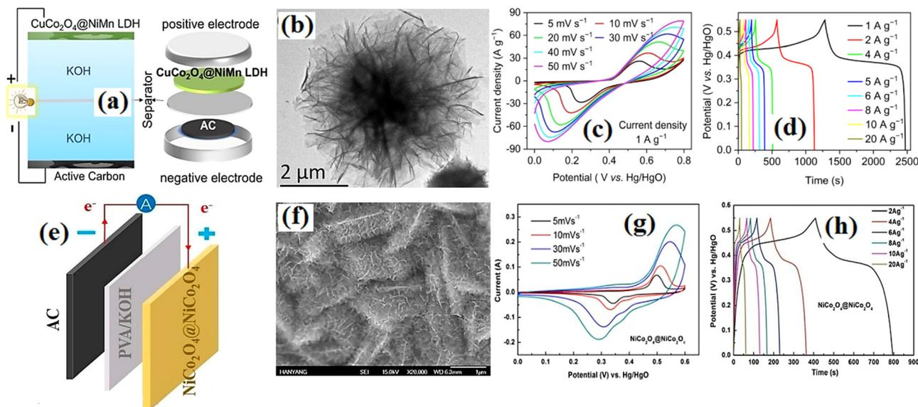
Fig. 11 (a) Graphical structure. (b) TEM image. (c) C–V curves. (d) Discharge curves of  $\text{CuCo}_2\text{O}_4@NiMn$  LDH//AC supercapacitor.<sup>197</sup> (e) Graphical structure. (f) SEM image. (g) C–V curves. (h) Discharge curves of the  $NiCo_2O_4@NiCo_2O_4//AC$  supercapacitor.<sup>199</sup>
