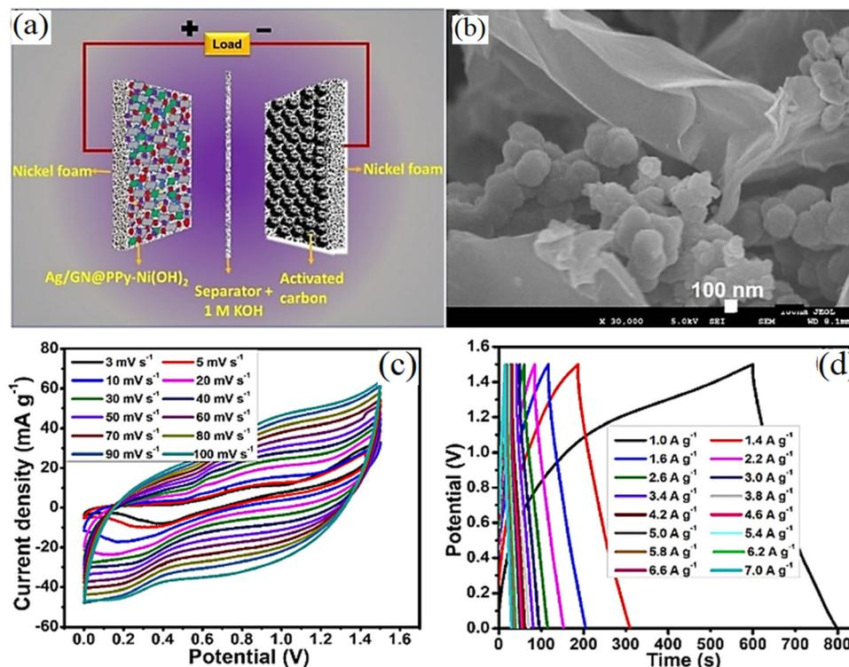
Fig. 8 (a) Schematic of supercapattery structure. (b) SEM image. (c) C–V curves. (d) Discharge curves of the Ag/GN/PPy–Ni(OH)<sub>2</sub>//AC supercapattery.<sup>138</sup>
